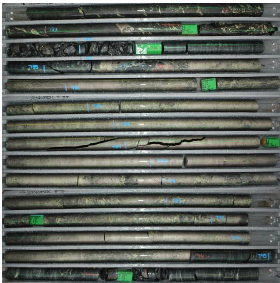
Figure 3. Composite image showing a high grade intercept from recent Great Cobar drill hole DD20GC0023C, comprising massive chalcopyrite-pyrrhotite-magnetite mineralisation and grading 11.7 metres at 4.4% Cu.
